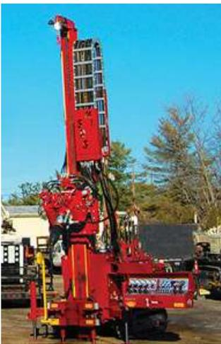
*Drill rig used to collect soil*
